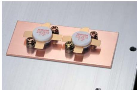
Copper Thermal Bonding Plate for Improved Dissipation
